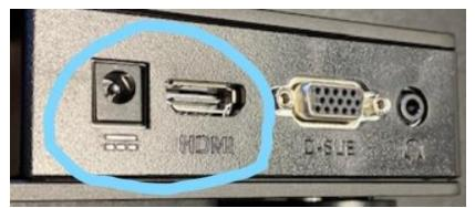
f.) Plug the power cable in blue into the round port and the HDMI cable in Red into the Red port. Each are keyed and should only go in one way. (See Picture)
