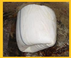
MPC ToughTube® can be designed to restore the full structural strength of the host pipe or it can be designed strictly as a liner depending on the degree of host pipe deterioration. It is available in a wide variety of shapes and pipe diameters from 6 inches to over 96 inches.
